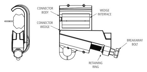
\* Not rated for HT Conductors
